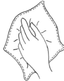
Wipe surfaces clean of dust and dirt. If in doubt, degrease using our Surface Preparation Wipes. (Isopropyl alcohol and water mix)
